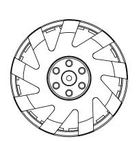
2X 90° PATTERN THREADS M2.5 x Ø 19mm M3 x Ø 19mm M3 x Ø 19mm
