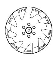
2X 90° PATTERN THREADS M2.5 x Ø 19mm M3 x Ø 19mm M3 x Ø 19mm [2.013] 51.12 [.745] 18.93 Ø 45.28 WIRES EXIT HERE
